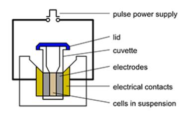
Electrical pulse creates temporary pore in membrane
