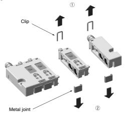
To remove the station, follow the same procedure for assembly and disassembly.
