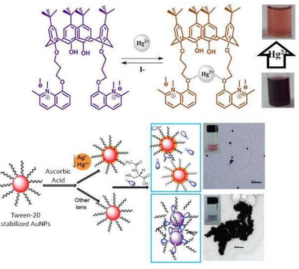
Functionalized nanoparticles can indicate metal concentration through color changes
