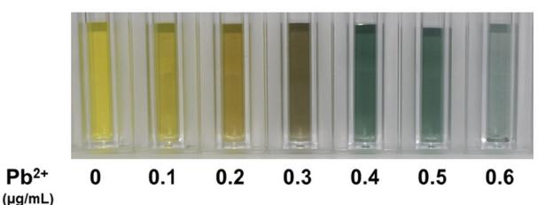
Organic colorimetric measures rely on characterized chemical reactions to determine metal presence
