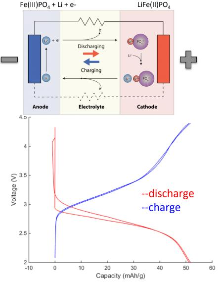
Theoretical capacity is 178 mA\*h/g value based on the reduced state of the cathode material - LiFe(II) $PO_4$
