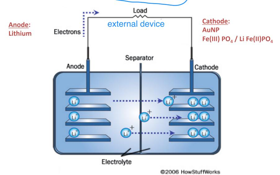
discharge: electrons flow from anode to an external load through the external circuitry to the cathode, "use of the battery"
